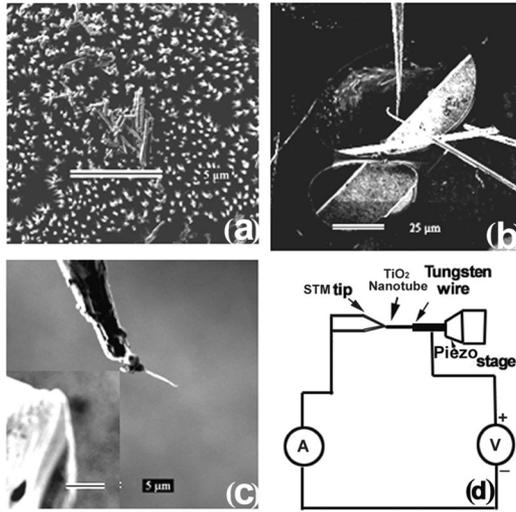
FIG. 2. Images from the FIB system show (a) the as grown TiO<sub>2</sub> nanotube sample; (b) FIB probe attached with a single nanotube, dispersed on the Cu mesh; (c) the FIB probe with a nanotube approaching the tip of the tungsten wire and; (d) schematic of the experimental setup for current-voltage measurement.
