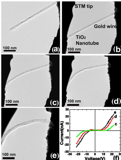
FIG. 3. (Color online) The bright field image of the TiO<sub>2</sub> nanotube (a) approaching the STM tip; (b) in contact with the STM tip; [(c)–(e)] undergoing a gradual increase in its bending curvature; (f) a series of the representative  $I$ - $V$  curves measured during the deformation of the TiO<sub>2</sub> nanotubes.
