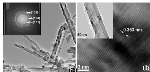
FIG. 1. (Color online) (a) An overall view of the anatase titania nanotube and the corresponding diffraction pattern (inset) and (b) the high resolution lattice image from a single anatase nanotube (inset).
