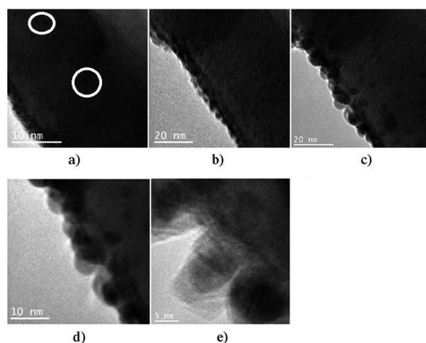
**Figure 5.** TEM images showing the decomposition of a ZnTe nanowire ( $d = 100$  nm,  $L = 200$  nm) with a 10 V bias. a) Onset of decomposition at 240 s; b) after 280 s; c) and d) growth of Zn and Te balls (grey and black) after 480 s; and e) surface of the nanowire after the evaporation of Zn and Te balls. The circles highlight the presence of the balls. The video of this process is available in the Supplementary Information.
