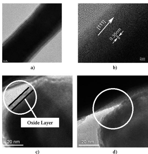
**Figure 4.** a, b) TEM images showing a thin oxide layer on the nanowire. The lattice spacing is 0.35 nm for the grown ZnTe nanowire and growth is along  $\langle 111 \rangle$  direction. Scale bars are 10 nm and 2 nm. c, d) Removal of the oxide layer with an STM bias of  $-10$  V (nanowire diameter = 70 nm). The bias-induced heating removes the oxide layer near the tip (area is marked by the circle).
