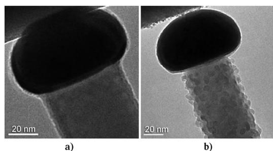
**Figure 6.** ZnTe nanowire with an intact gold catalyst particle at the tip. a) Before decomposition and b) 20 min after the onset of decomposition. The diameter in (a) is uniformly 58.4 nm, whereas in (b) the diameter differs along the stem with an average of 53.0 nm.
