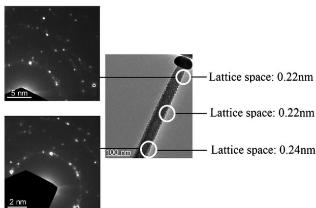
**Figure 8.** Lattice spacing and diffraction patterns at different spots on the nanowire.
