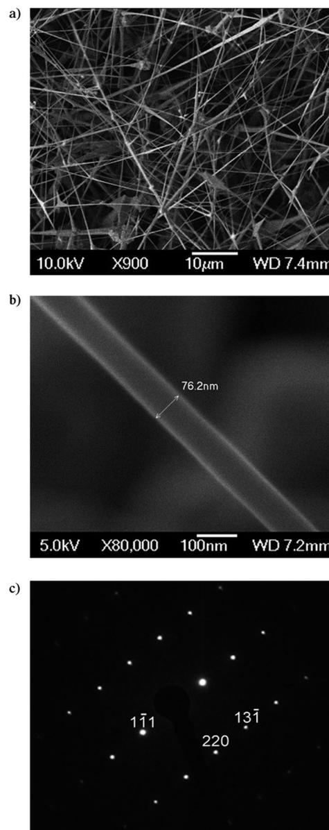
**Figure 2.** SEM images of a) a mat of ZnTe nanowires and b) an individual nanowire  $\sim 70\text{ nm}$  in diameter. c) SAED pattern of a grown ZnTe nanowire.
