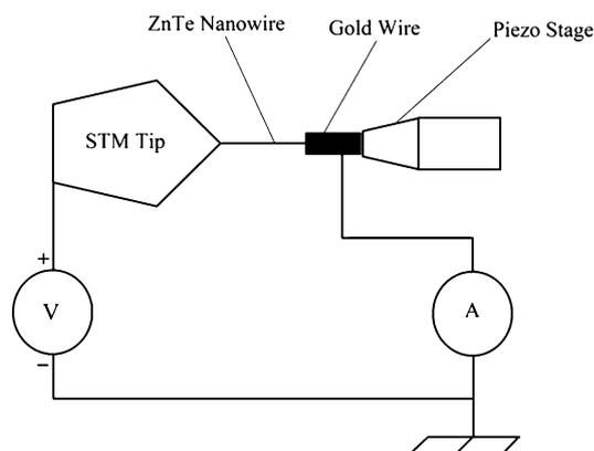
**Figure 1.** STM-TEM setup. An individual ZnTe nanowire is placed between the STM tip and a gold wire. The gold wire with the attached nanowire is placed on a moveable piezotube enabling 3D motion toward the STM probe.
