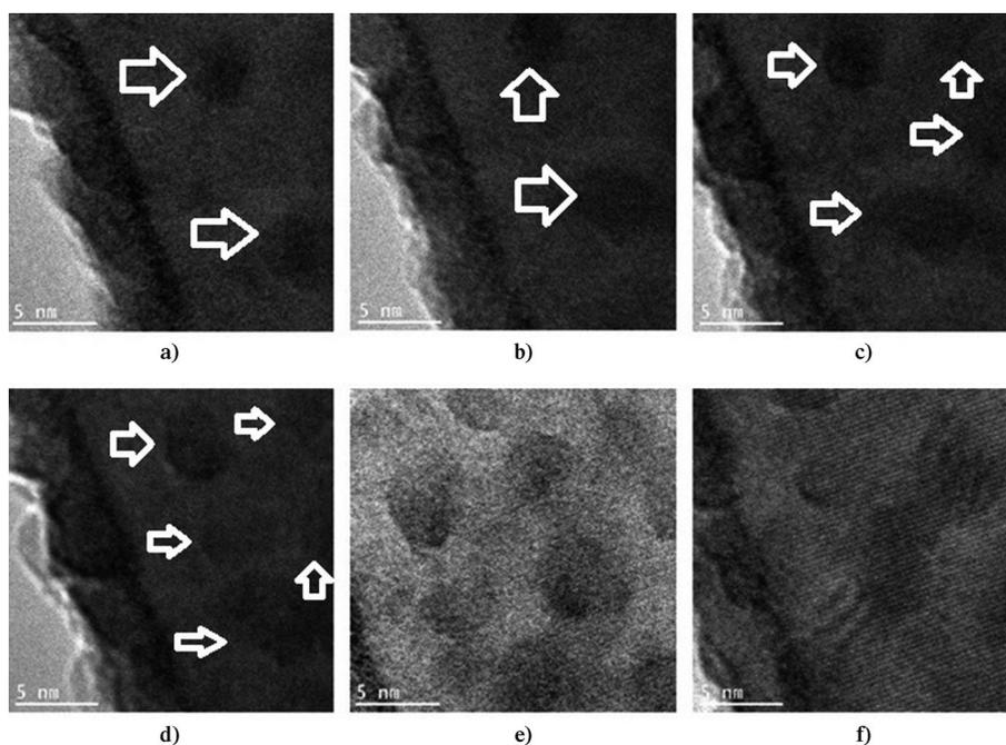
**Figure 7.** Zn and Te ball formation during the breakdown of the ZnTe nanowire shown in Figure 6. Because of the high magnification, the gold particle is not seen and only a portion of the nanowire is shown. a) After 5 min; b) after 7 min; c) after 8 min; d) after 11 min; e) after 15 min.; and f) after 20 min. The balls grow and aggregate. The arrows point towards the balls.
