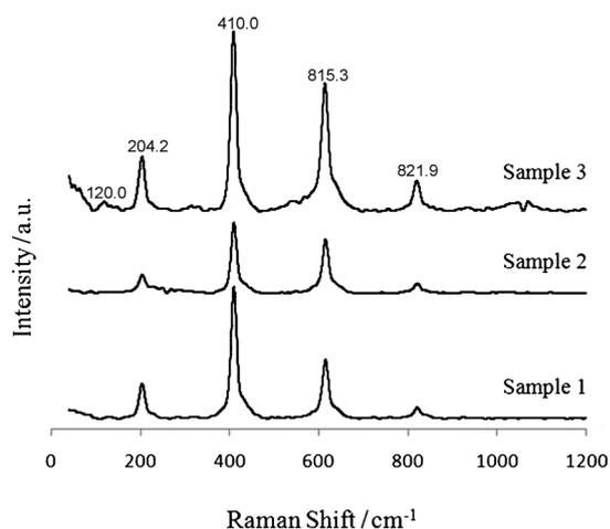
**Figure 3.** Raman spectra of three representative ZnTe samples. Growth conditions are identical to those described in the text except that Samples 1 and 2 were grown with flow rates of 150 sccm and 60 sccm. Sample 3 was synthesized with 900 °C as source evaporation temperature.
