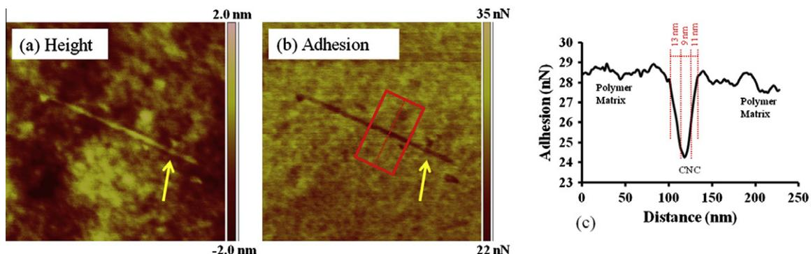
**Fig. 6.** (a) Height and (b) adhesion maps with size of  $1 \times 1 \mu\text{m}^2$  showing a single CNC (marked by yellow arrows). (c) Average adhesion profile of the area shown by red rectangle in adhesion map in (b). Using this profile, CNC diameter (9 nm) and average thickness of the interphase were measured. (For interpretation of the references to colour in this figure legend, the reader is referred to the web version of this article.)
