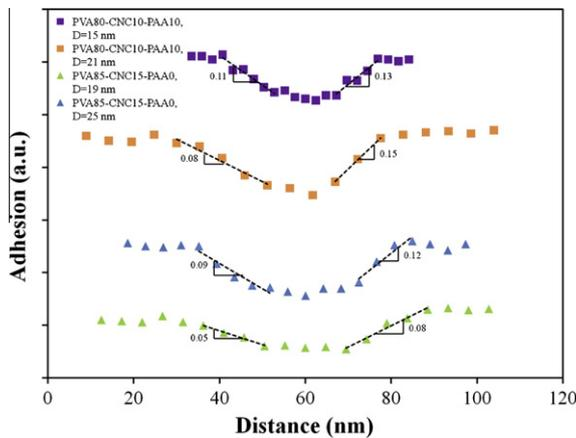
**Fig. 5.** Average adhesion profiles (arbitrary unit, a.u.) in PVA 80–CNC 10–PAA 0 (square) and PVA 85–CNC 15–PAA 0 (triangle) composites. Dashed lines were used to measure the rate of change in adhesion at the interphase ( $\text{nN nm}^{-1}$ ).
