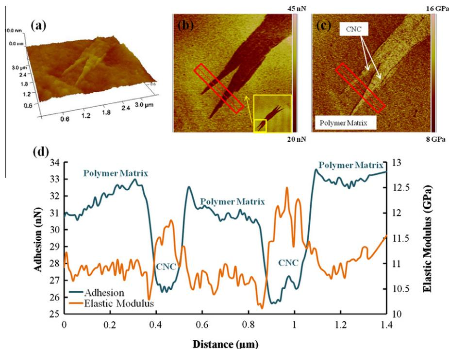
**Fig. 3.** (a) 3D height, (b) adhesion, and (c) elastic modulus maps ( $3.5 \times 3.5 \mu\text{m}^2$ ). Inset in (b) shows the scanning area (PVA 80–CNC 10–PAA 10). (d) The average adhesion and elastic modulus profiles of the area in the red boxes in (b) and (c). Polymer matrix and CNC regions are marked on the profile. Interphase region is the distance that adhesion and modulus profiles are overlapped.
