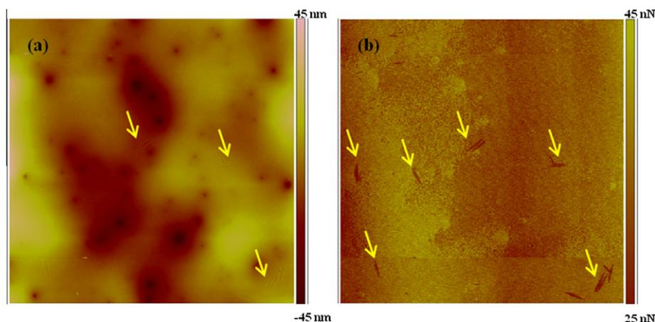
Fig. 2. (a) Height and (b) adhesion maps of a 50 × 50 μm<sup>2</sup> region on a PVA 80–CNC 10–PAA 10 sample. The arrows point to CNCs embedded in the polymer matrix. The presence of CNCs is easily distinguishable from the adhesion image.
