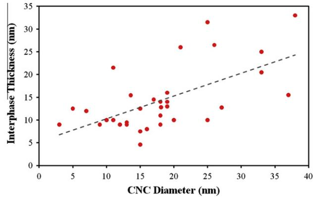
**Fig. 7.** Change in interphase thickness with CNC diameter. Red circles show average interphase thickness of the CNCs. The trend line (dashed gray line) shows an increasing trend in the interphase thickness with the CNC diameter. (For interpretation of the references to colour in this figure legend, the reader is referred to the web version of this article.)
