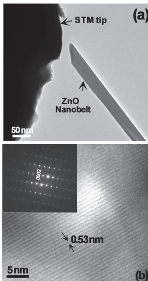
**Figure 1.** (a) A ZnO nanobelt and its (b) corresponding electron diffraction pattern (inset) and the high-resolution lattice image.
