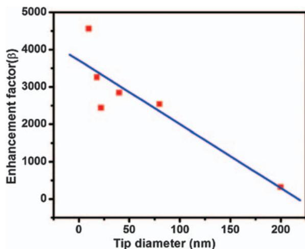
**Figure 4.** The variation of field enhancement factor,  $\beta$  with the tip diameter of the nanobelts.
