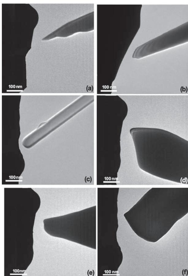
**Figure 2.** The bright field images of the ZnO nanobelts with different tip shape and width,  $w$  ranging from 10–200 nm.
