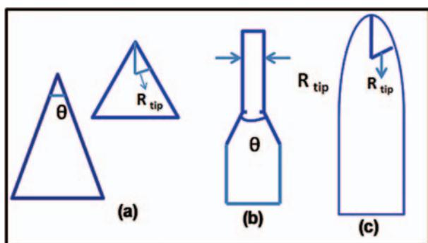
**Figure 5.** Schematic diagram presenting the shape of the tip of the nanobelts (a) agave like (b) pencil like (c) round structure.
