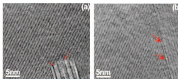
**Figure 6.** HRTEM image of the tip of the nanobelt. The planar defects in the image are marked by red arrow.
