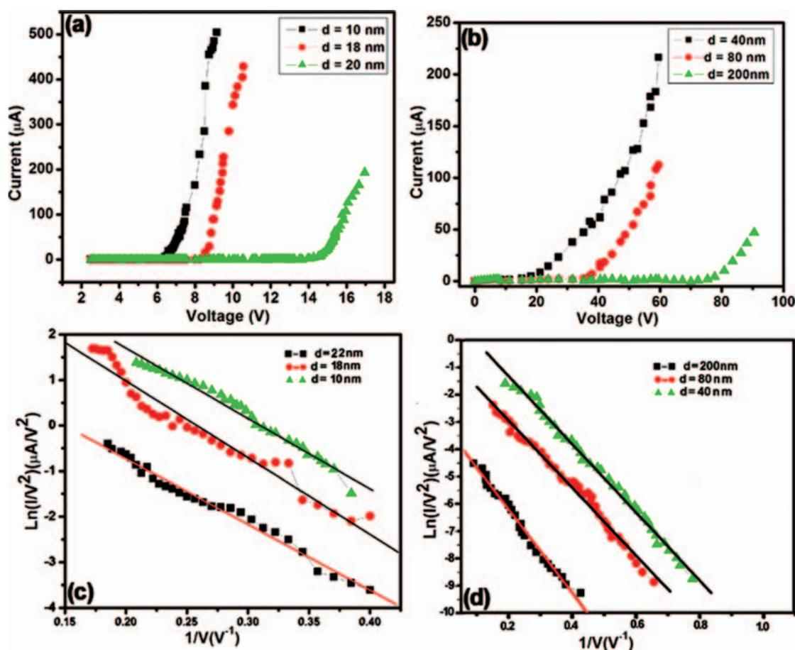
**Figure 3.** (a) The  $I$ - $V$  curves of the nanobelts having width,  $w \sim 10, 18$  and  $22$  nm. (b)  $I$ - $V$  curves of the nanobelts having  $w \sim 40, 80$  and  $200$  nm. (c) The  $F$ - $N$  plots of the nanobelts having  $w \sim 10, 18$  and  $22$  nm and (d) The  $F$ - $N$  plots of the nanobelts having  $w \sim 40, 80$  and  $200$  nm.
